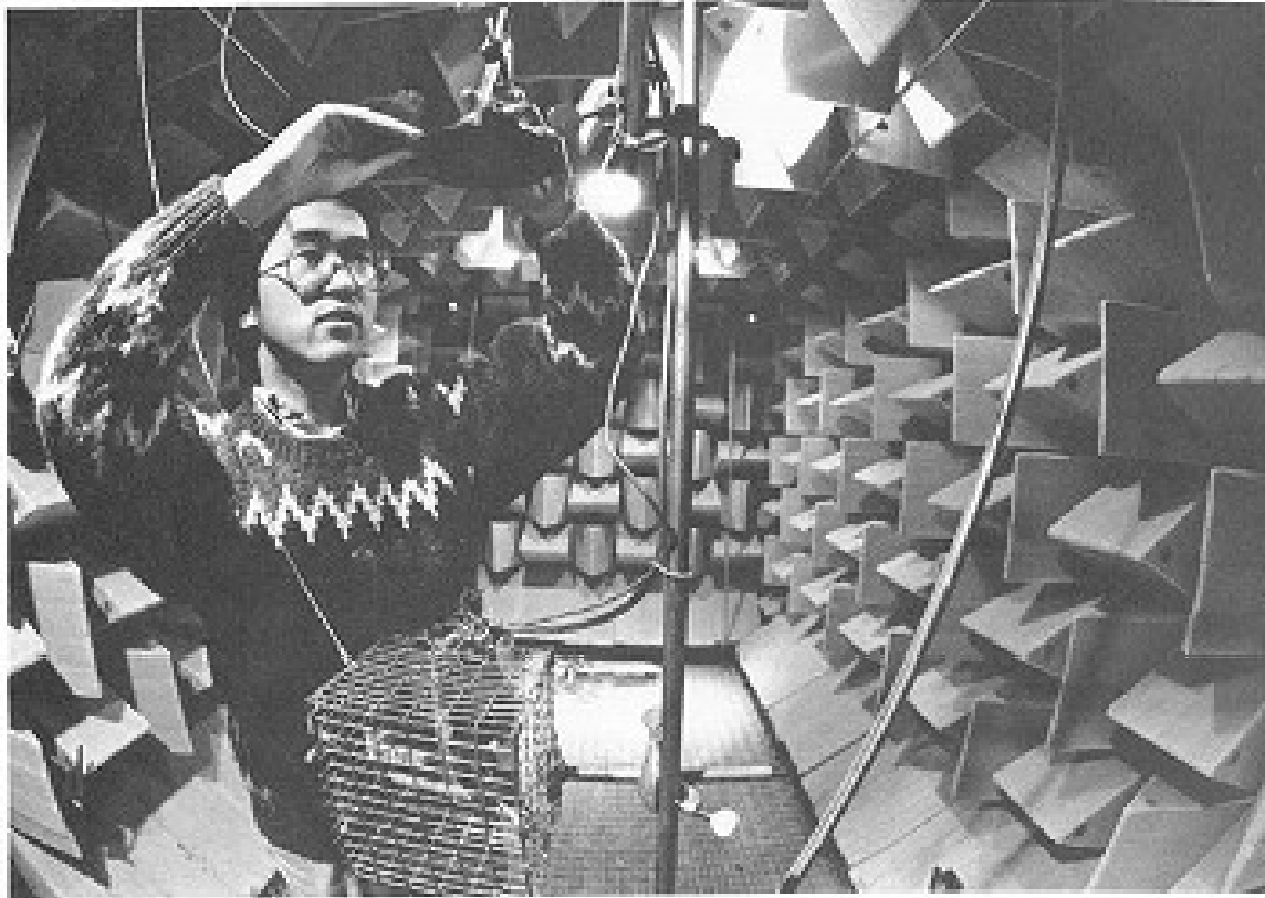
UMCP psychology graduate student Kazuo Okanoya adjusts a speaker used to measure a canary's threshold of hearing in an anechoic chamber.
